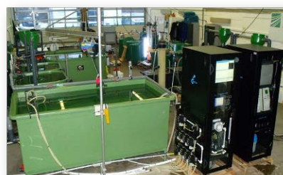
OceanPack Aquaculture IMTA system water quality monitoring for 20 tanks with water supply control, e.g. CO 2 , nutrients, oxygen; incl. auto-cleaning
