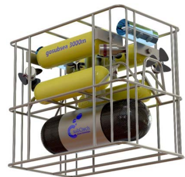
Underwater vehicle for offshore construction monitoring
